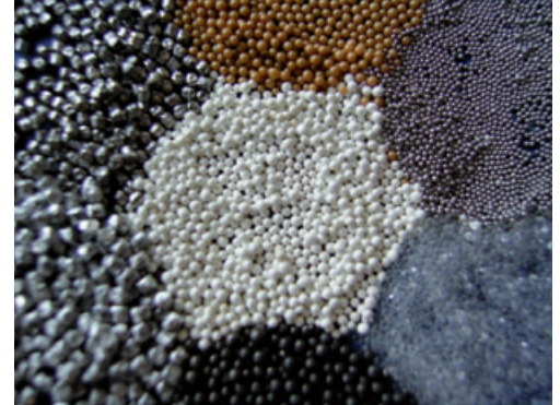
Blasting medium: cut wire shot made of stainless steel
